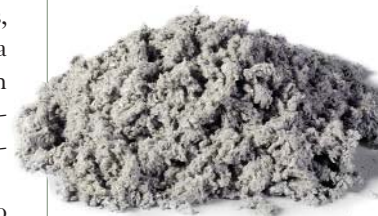
Cellulose is made from recycled paper.
