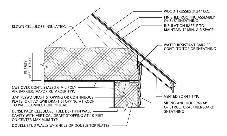
Double Stud Wall: Roof Connection
