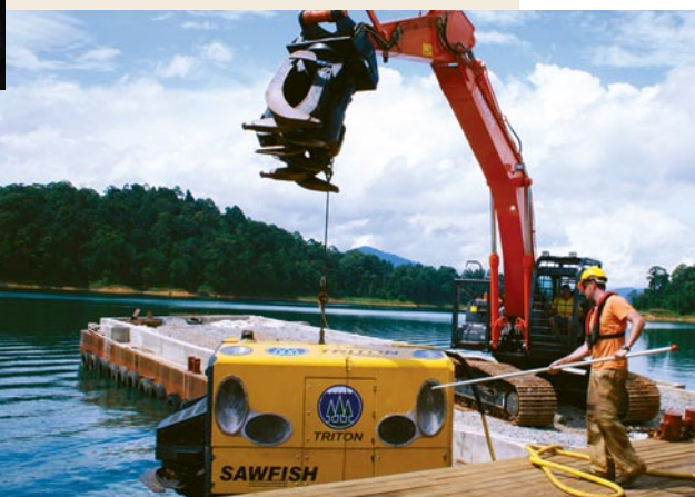
New school. The remotely operated Sawfish clears standing timber flooded by dam projects. The submersible can operate hundreds of feet down.
