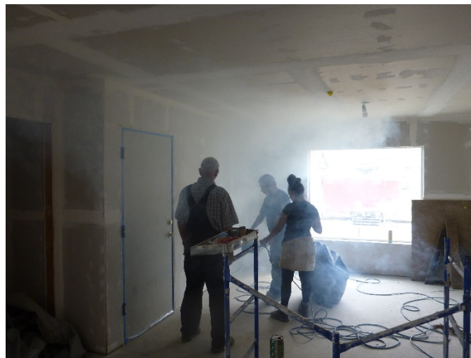
Figure 10. Smoke Test in House 9 (Chitwood Energy Management)
